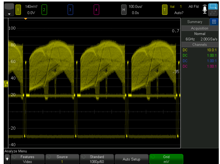
Figure 45. Triggering on a 1080p/60 signal.
