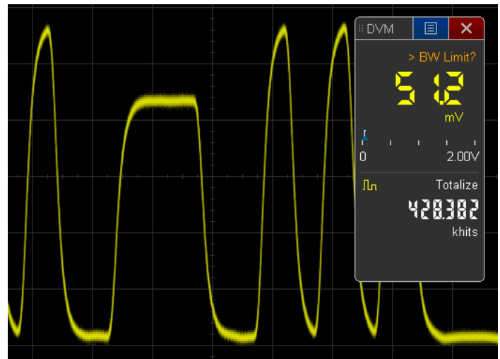
Figure 35. Totalizing the number of runt errors.
